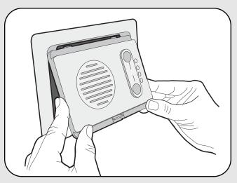
Place intercom in frame by inserting top section first, then snapping the lower section into place.
